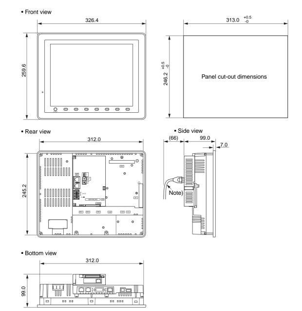
2-2-1 External dimensions and panel cut-out dimensions for the NP5M0101-5H4/NP5N0011-5H4 (Unit: mm)
